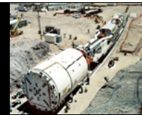
Yucca Mountain TBM 90's model Electric and 450ft long. It only took 10 months to build the Yucca Project TBM
