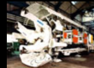
Mobile Tunnel Miner (MTM) An undercut borer with adjustable jaws. (hard rock)
