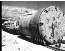
60's model (Electrically Powered) Same company built Yucca TBM (Construction & Tunneling Services, Inc.)
