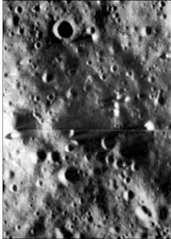
Figure 11 Shaded image computed from DEM based on a Lambertian surface reflectance function. Similarity to image in Figure 8 validates accuracy of DEM.
