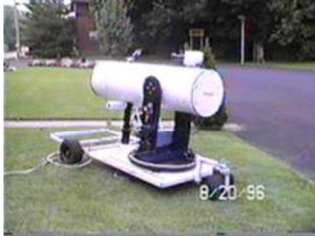
Figure 1 16" Newtonian telescope mounted on Scope Transport Unit.
